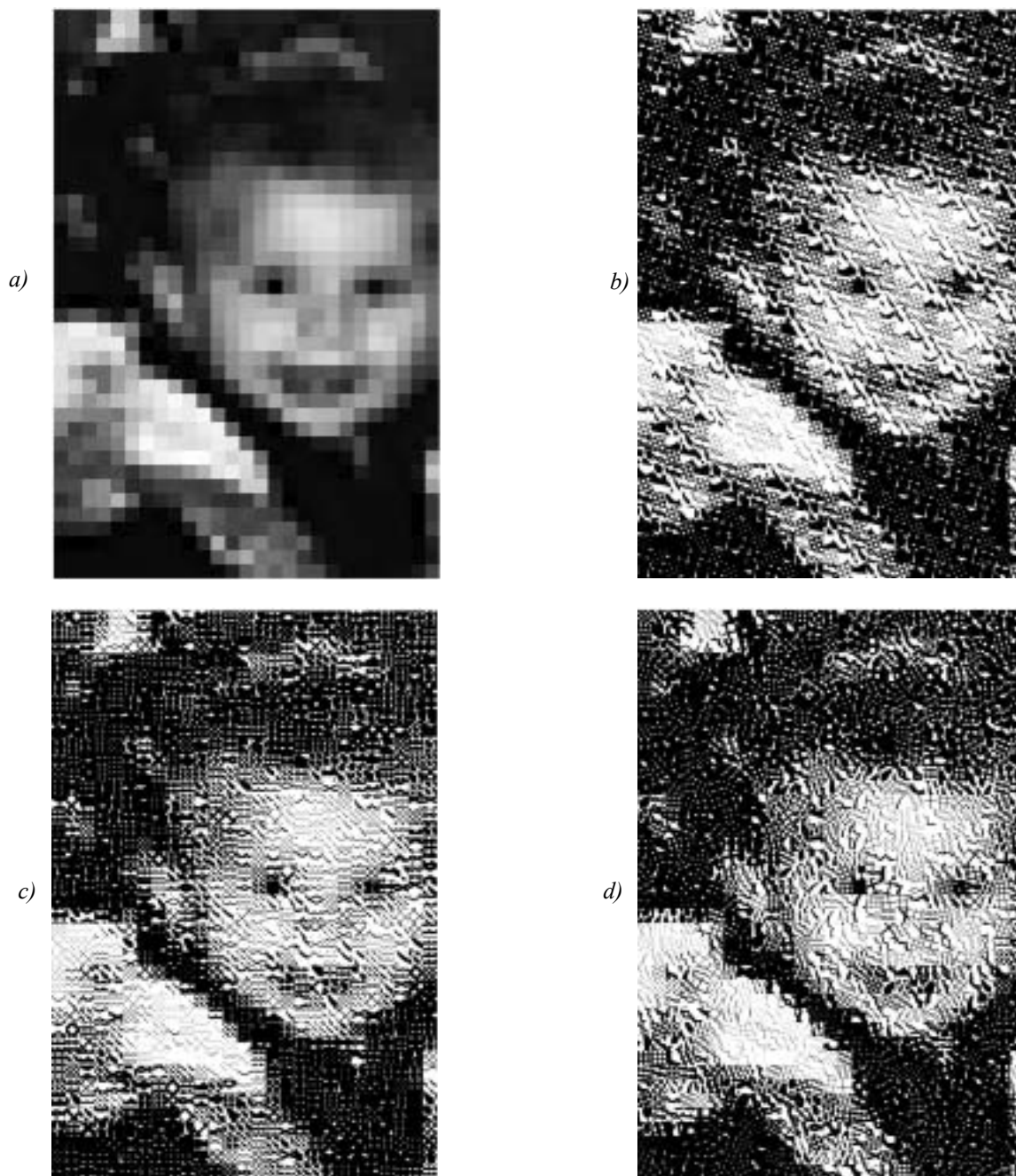
Fig. 54 a) standard dot halftone screen b) screening with cyclic continuity of screening algorithm c) screening with stochastic selection of halftone screen element shape algorithm (SEED = 12345678) \alpha = 0^\circ d) screening with random selection of halftone screen element algorithm and random selection of screening angle \alpha (SEED = 246135)
