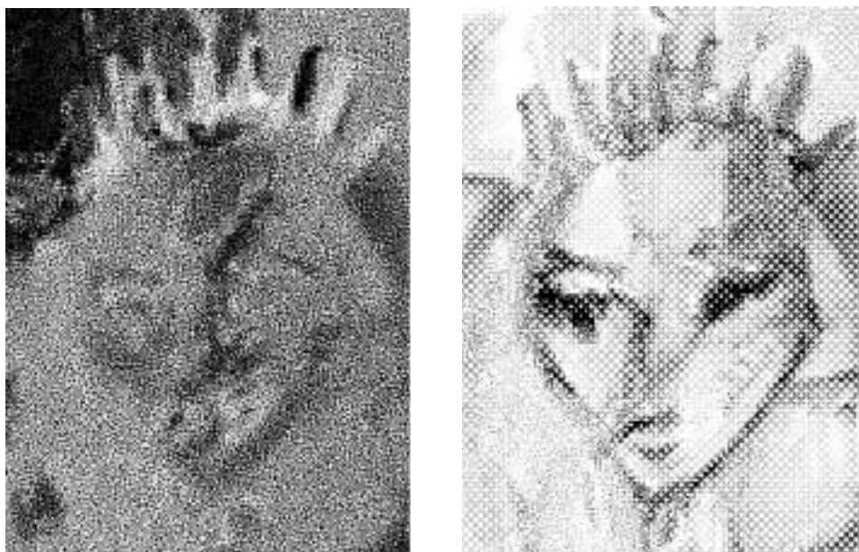
Figure 68 'Maska', yellow and black channels, ring screen shape in low gray levels in yellow color
